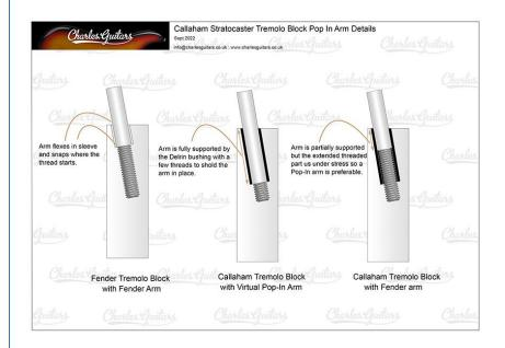
All Callaham blocks come with a precision-reamed Delrin insert in the arm hole, allowing the tremolo arm to fit snugly and be free of play, without requiring a spring in the hole as Fender's threaded blocks do. This gives you the best tremolo feel available, and no worries about losing springs (in case you're unaware of it, new Stratocasters ship with a round label over the hole in the tremolo - the label's purpose is to prevent the tiny spring from falling out and being lost).
