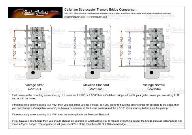
Fender has used a couple of dimensions over the years for both string spacing and screw spacing on tremolos. The drawing shows you the differences between the various bridges, so you can be sure of getting the right fit. You can click the image to download a PDF that is to scale.
